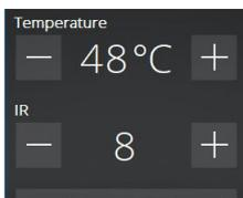
When the set temperature is 40 °C, the sauna heater will not heat the sauna and only the infrared heaters will be active. The infrared heaters remain active for different lengths of time depending on the IR scale step (see table). If the temperature is set to between 41 and 60 °C and the set temperature has not been reached, two of the heating elements will heat up when the infrared elements are active.
