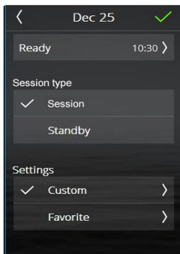
"Ready" means that the system learns how long it takes to heat the room to the desired temperature. It does this by calculating the number of degrees by which the temperature increased per minute the last five times it ran. During the first five times the system runs a default value is used for temperature increase, but after this the calculated value for the relevant room is used.
