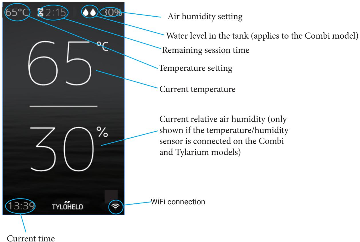
If a calendar program or weekly program is about to start, the screen will switch on about one hour before this and the following Overview screen will be displayed:
