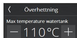
In steam generators, the maximum temperature setting in the water tank applies. If the temperature is exceeded, the water tank will be emptied. If the water temperature reaches this temperature, it is probably because the water quality has deteriorated to the point where the water is foaming. In this situation the heating element is at risk of damage.
