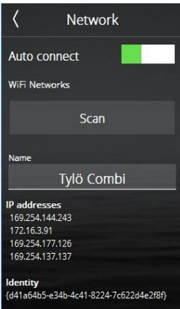
Bear in mind that the position where the control panel is located affects how well it can communicate with the wireless network. Many kinds of material disturb the Wi-Fi signal. stem and go into Network. Available networks will be displayed with a relative signal strength indicated in % after each name. The signal strength must be at least 60% or you risk losing the connection. If the signal strength is less than 60%, a new access point or repeater must be installed near the Elite panel. .
