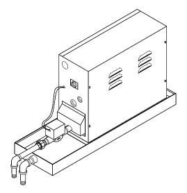
Connect appropriate 1/2" drain pipe to generator drain valve. DO NOT drain water from generator drain valve directly into drip pan.
