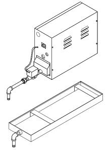
Screw suitable pipe adapter into 3/4" female NPT threaded outlet in pan and connect to a plumbing system drain line.
