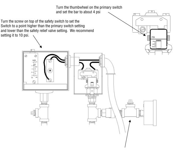
A fitting is supplied to allow connecting a second pressure gauge to easily replace the supplied gauge or to connect a second gauge for inspection. A ball valve is supplied assist with gauge changes; the valve should be left open during normal operation.
